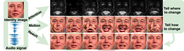
Figure 1: Problem description. The model takes an arbitrary audio speech and one face image, and synthesizes a talking face saying the speech.
