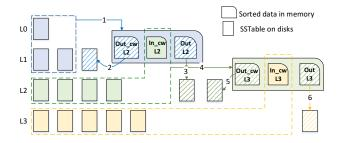
Figure 8: **Process of gear compaction.** The active compaction of  $L_0$  and  $L_1$  drives passive compactions in higher level. The resultant data of each compaction is divided into three parts according to its key range, including out of  $L_i$ 's compaction window (Out\_cw  $L_i$ ), in  $L_i$ 's compaction window (In\_cw  $L_i$ ), and out of  $L_i$ 's key range (Out  $L_i$ ).
