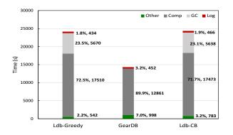
Figure 14: **Random load time breakdown.** This figure shows the time spent (the y-axis) on different operations when we randomly load an 80 GB database. The numbers next to each bar show their time consumption and the ratio to the overall run time. For LevelDB, compaction and garbage collections take the most significant percentage of the overall runtime. GearDB eliminates the garbage collections and improves compaction efficiency.
