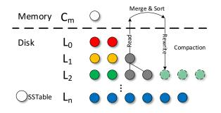
Figure 1: A compaction process in an LSM-tree based KV store. This figure shows the LSM-tree data structure, which is composed of a memory component and a multi-leveled disk component. Compaction is conducted level by level to merge SSTables from the lower to higher levels.
