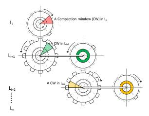
Figure 9: Compaction windows are reclaimed in a gear fashion. The red, green, and yellow sectors represent the compaction windows of  $L_i$ ,  $L_{i+1}$ , and  $L_{i+2}$ . Compaction windows are reclaimed by compaction like a group of gears. Reclaim k compaction windows (CW) in  $L_i$  mimics a full round moving of a gear, which leads to one move in the driven gear, that is cleaning one compaction window in  $L_{i+1}$ , and so on.
