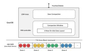
Figure 6: **The architecture of GearDB.** *This figure shows the overall structure of GearDB with three design strategies. GearDB accesses the HM-SMR drive directly via the T10 zone block command. For the data layout on an HM-SMR drive, SSTables form the same level are located in integral zones, and each zone only serves SSTables from the same level.*  $\bigcirc$  *represents the SSTable from L<sub>i</sub>.*
