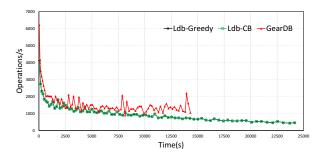
Figure 11: **Detail of random load.** This figure shows the incremental performance of every 1 GB randomly loaded during the process of loading an 80 GB database. GearDB has higher throughput and a shorten execution time for loading the same sized database compared to LevelDB.
