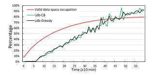
Figure 3: **Cost of garbage collections.** *The green line shows the ratio of valid data volumes to the test disk space; the other two lines show the ratio of time consumption of garbage collections in every ten minutes during the random loading.*
