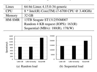
Figure 10: Load performance. GearDB shows its advantage in both random load and sequential load compared to LevelDB.
