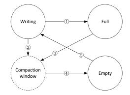
Figure 7: **Zone state transitions in GearDB.** In GearDB, multiple zones are allocated to each level according to the data size of that level. These zones can be in three states during their lifetime, namely writing zone, full zone, and empty zone. Zones, including full zones and writing zones, rotate to construct a compaction window.
