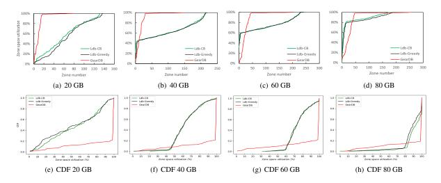
Figure 17: **Zone space utilization.** *Figures a-d show the zone space utilization of each occupied zone when we randomly load* 20, 40, 60, and 80 GB database. Figures e-h show the corresponding CDF of the zone space utilization. The results show that our design consistently maintains a high space efficiency.
