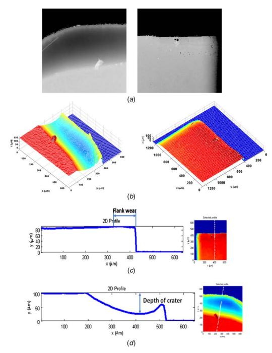
Fig. 6 Tool wear analysis with 3D confocal images: (a) HEI image, (b) 3D confocal image, (c) 2D profile of flank wear, and (d) 2D profile of crater wear
