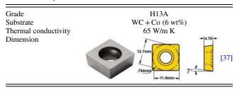
the carbide grains is 1  $\mu$ m, do not have any chip breaker to minimize the cutting temperature variations on the rake face. The detailed specification of the insert is given in Table 2.<sup>3</sup>
