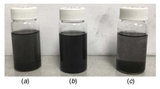
Fig. 3 Stability in mixtures of oil: (a) 0.1, (b) 0.5, and (c) 1.0 wt% xGnP M5 after 72 h
