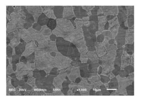
Fig. 1 Microstructure of Ti-6AI-4 V in the STA condition
