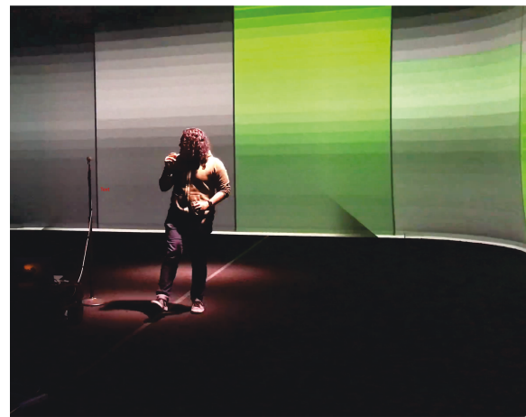
Fig. 4: Tracking and integration test. The location estimate of the author is broadcast to a lighting array and browser-based application, visually highlighting the author's position.
