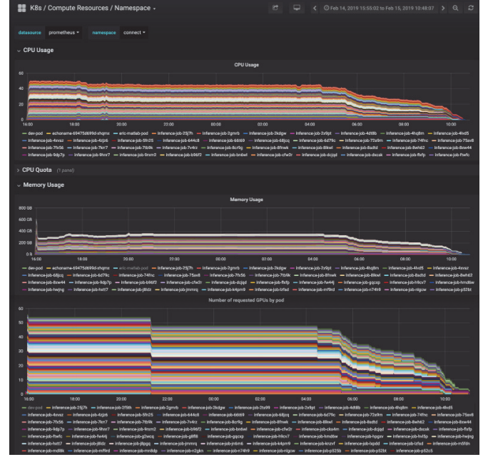
Fig. 6. Inference job - Top) Number of CPUs being utilized, Middle) Memory utilization, Bottom) Number of GPUs being utilized.
