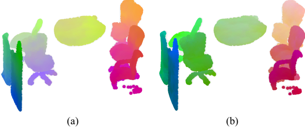
Figure 3. A visualization for the learned instance sensitive features. (a) shows the context features f_c by first applying PCA to the high dimensional features and then converting the first three dimension into the color map here. (b) shows the predicted object centers. A clearer separation of different instances is shown in (b), which confirms that these features are instance sensitive.
