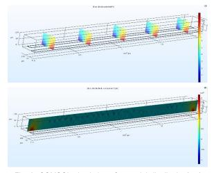
Fig. 2. COMSOL simulation of potential distribution(top) and electric field distribution (bottom) of the interdigitated electrode array.
