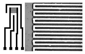
Fig. 1. (left) Schematic drawing of electrode with interdigitated design. (right) Micrograph of the interdigitated electrode arrays (IDEAs) used in the experiments. The width of the electrode is 40 microns.
