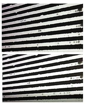
Fig. 5. The mix of 1  $\mu$ m and 5  $\mu$ m diameter beads is separated under the influence of 10 kHz, 3Vpp, 1V offset bias. The images (top and bottom) were captured 2 seconds apart. Smaller beads experience pDEP and are attracted to the electrode fingers (seen as small protrusions along the edges of the electrodes), while larger beads move to the left side of microelectrode array.
