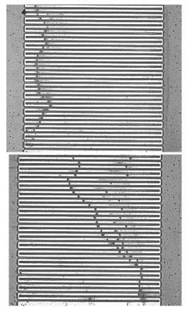
Fig. 4. 1  $\mu$ m beads under the influence of 100 KHz,3 Vpp bias move to the left edge of the electrode array when the offset is + 1.3V (top), but movement of the beads switches to that towards the right edge when the offset is changed to -1.3Vpp (bottom).
