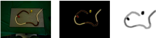
Fig. 6. Preprocessing procedure. Image 1: original photo as seen by the PR2, Image 2: background removed from image, Image 3: Preprocessed to have one color channel
