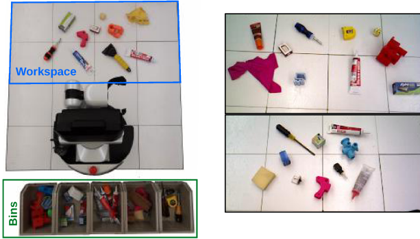
Fig. 7: Left: Top view from setup for surface decluttering experiment. Right: Two sample input images taken from the experiment.
