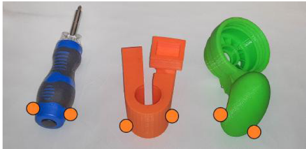
Fig. 8: Three example failure modes from Dex-Net MM. Left: The object was lifted successfully, but the screwdriver’s weight caused it to rotate and then it slipped out of the gripper during transportation. Center: The robot grasped slightly more below than planned and the object slipped because of the round surface. Right: Due to motion imprecision, the HSR grasped further below than planned and failed to grasp the object. Such counter examples may be due to limited positive grasps.
