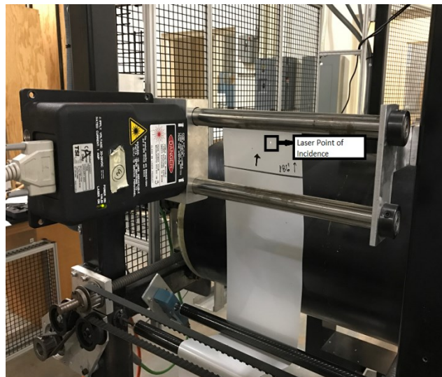
Figure 3 – LDV setup at winder entrance
