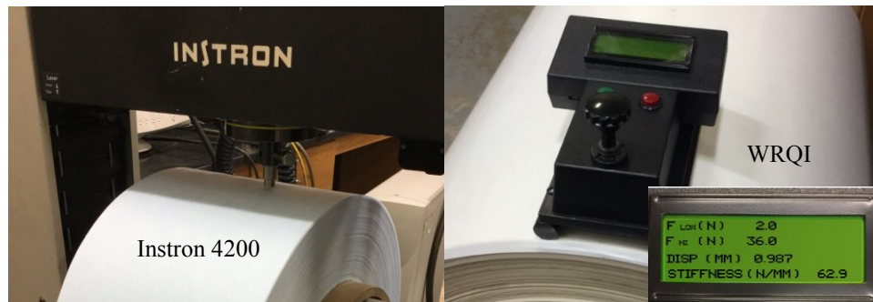
Figure 3 – Surface Stiffness Testing Instruments: Instron 4200 and WRQI
