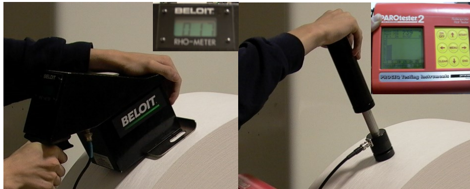
Figure 2 – Hardness Testing of a Wound Roll of Nonwoven
