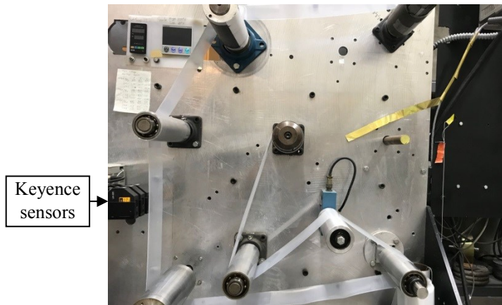
Figure 11 – On-line measurement of CMD Curl
