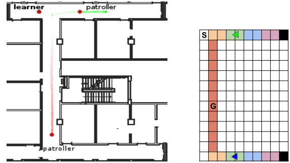
Figure 1: The map and the corresponding MDP state space for each patroller [4]. MDP has 3 dimensional state space (x, y, \text{orientation}) with 124 states, and it has 4 actions (move-forward, turn left, turn right, stop). The color-shaded regions (long hallway, turning points and 3 small divisions in small hallways on both sides) are the 5 regions defining movement and turn-around features. S and G are start and goal locations for the learner. Simulations were run on a Ubuntu 14 LTS system with an Intel i5 2.8GHz CPU core and 8GB RAM. Learner is unaware of where each patroller turns around or their navigation capabilities.
