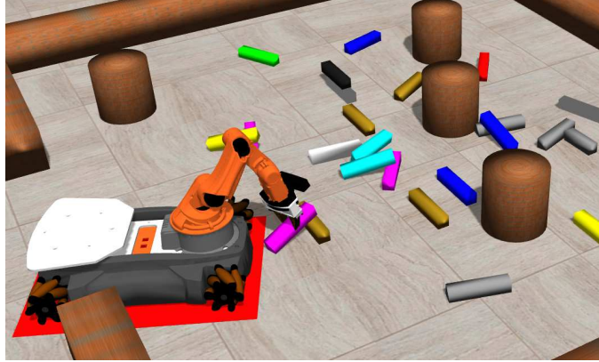
Fig. 1. A clutter removal scenario addressed in this work, where a KUKA youBot is tasked to grasp and remove all scattered objects in clutter, one at a time, in a room with four static obstacles.
