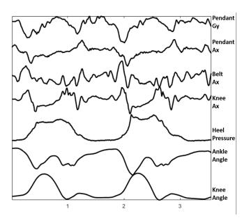
Fig. 4. The response of exoskeleton sensors while a volunteer was walking over ground.
