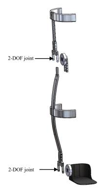
Fig. 1. Exploded view of 2-Degree-of-Freedom (DOF) joints of the Measurement exoskeleton system (developed for right leg)
