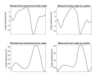
Fig. 5. A comparison of ankle and knee displacement angles measured by the exoskeleton system and standard biomechanical walking signal.
