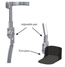
Fig. 2. Detailed view height adjustment mechanism
