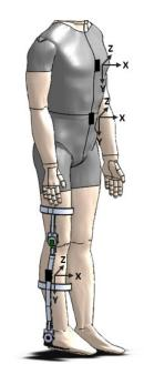
Fig. 3. An illustration of IMU placement with skeleton system
