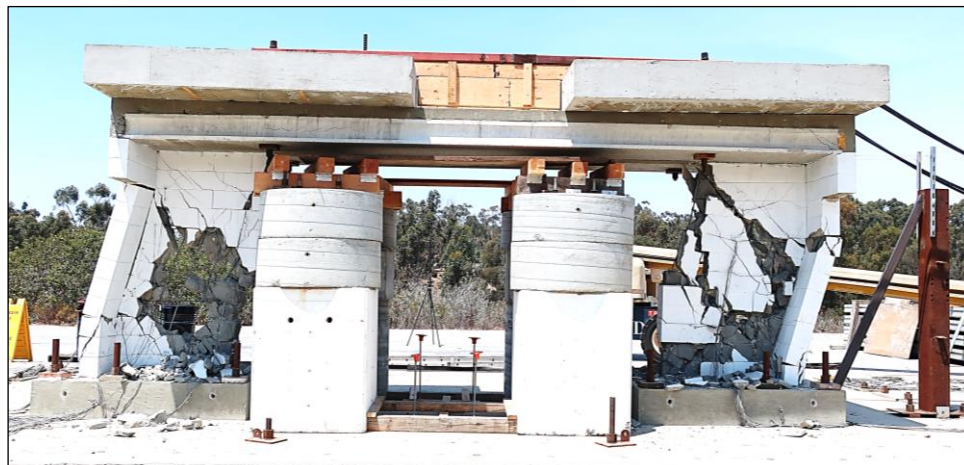
Figure 12. Specimen 1 after the static pull test
