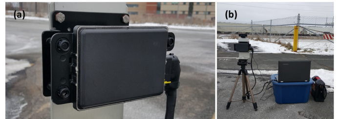
Fig. 9. (a) Delphi ESR, and (b) Experimental setup using a tripod.
