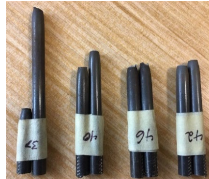
FIGURE 17. Fractured specimen for thick (37 and 46) and thin (40 and 42) samples from pulsing experiments
