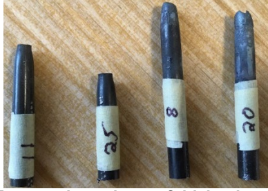
FIGURE 2. Fractured specimen of thick tube samples with current density of 0, 6.8, 10.5 and 13.7 A/mm 2 (left to right)
