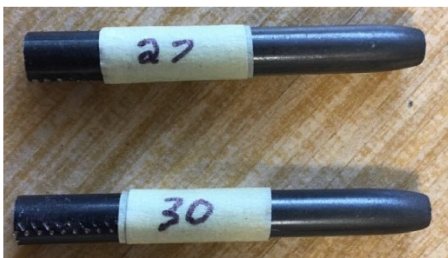
FIGURE 12. Fractured specimen for thin samples with 5 and 50 mm/min
