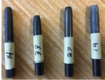
FIGURE 3. Fractured specimen of thin tube samples with current density of 0, 6.8, 10.5 and 13.7 A/mm 2 (left to right)
