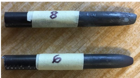
FIGURE 11. Fractured specimen for thick samples with 5 and 50 mm/min
