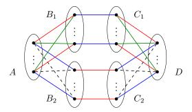
Fig. 5. The blue and red edges represent the matching picked at rounds 1 and 2, respectively. The green edges represent the edges picked at round 3 and above. The dashed edges are never picked by the algorithm.
