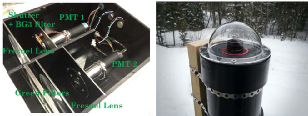
Figure 7.25 Optical instruments: the Stanford large-aperture photometer (left) and an all-sky imager (right).
