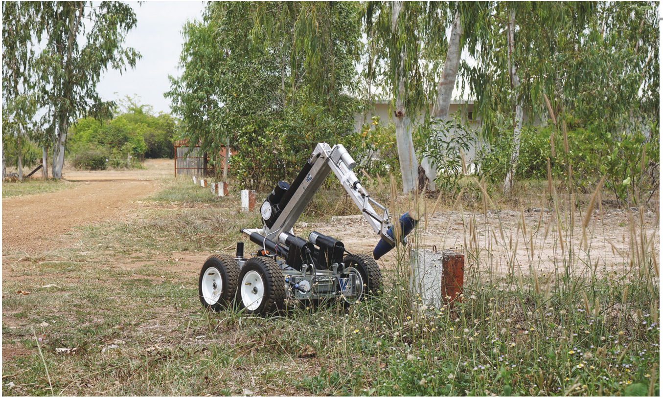
FIGURE 1 The VU-GWHF EOD robot performing a simulated EOD mission. Photo taken at the GWHF test facility in Kampong Chhnang, Cambodia.
