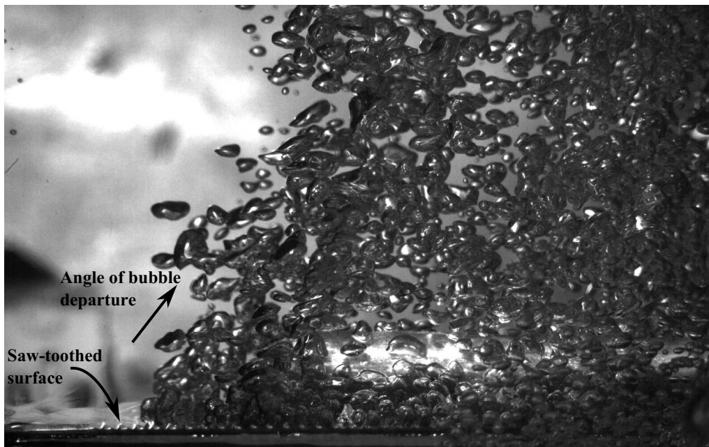
FIG. 5: Image showing bubble departure from re-entrant cavities at an angle normal to the sloped surface of the ratchets during saturated pool boiling at a heat flux of 2.2 \text{ W/cm}^2 .
