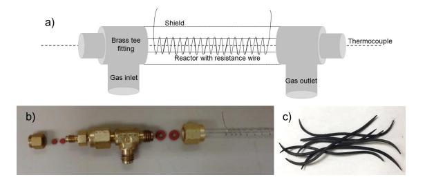
**Fig. 1.** a) Schematic of reactor setup. The quartz reactor was wrapped with a resistance wire and surrounded by a silvered borosilicate shield. Three-way fittings on the ends allowed gas flow in or out, and provided thermocouple exits; b) One end of reactor was setup with fittings, o-rings, reactor, and resistance wire; c) Sample of biochar stock used in each reaction - only a small ~4 mg piece of this biochar was actually used in a given experiment
