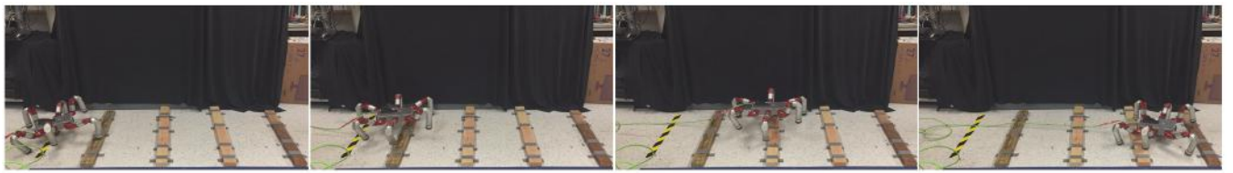
Fig. 9. The figure shows the hexapod attempting to cross obstacles using the CPG parameters learned for obstacle height 5cm to cross obstacles of height 5cm. We see that the robot easily makes past all the obstacles in front of it.
