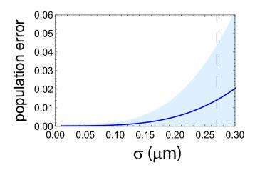
FIG. SM-2. Numerical solutions for the population error due to atom position variations after a  $\pi$  ground-Rydberg pulse with  $\pm$  one standard deviation shown by the light blue shading. The vertical dashed lines show the expected value of  $\sigma$ . All other parameters the same as in Fig. SM-1.
