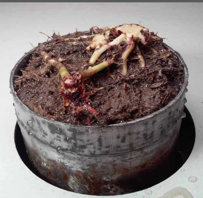
Figure 1: A) Sorghum Sample before Erosion Test; B) Sorghum Sample after Erosion Test; C) Erosion Function Apparatus
