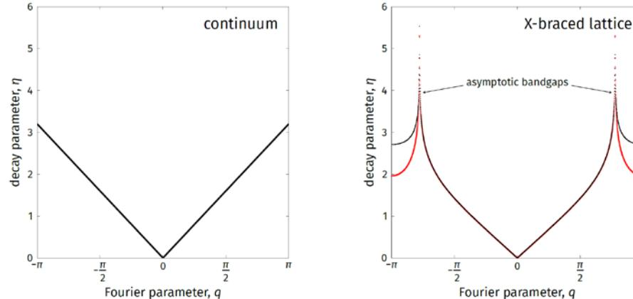
Coarseness or fineness of applied surface strain is measured by the Fourier parameter, the wavenumber  $q$ . Low  $q$  corresponds to coarse surface excitations while high  $q$  corresponds to fine surface excitations. The rate at which a static mode of deformation decays with distance is defined
