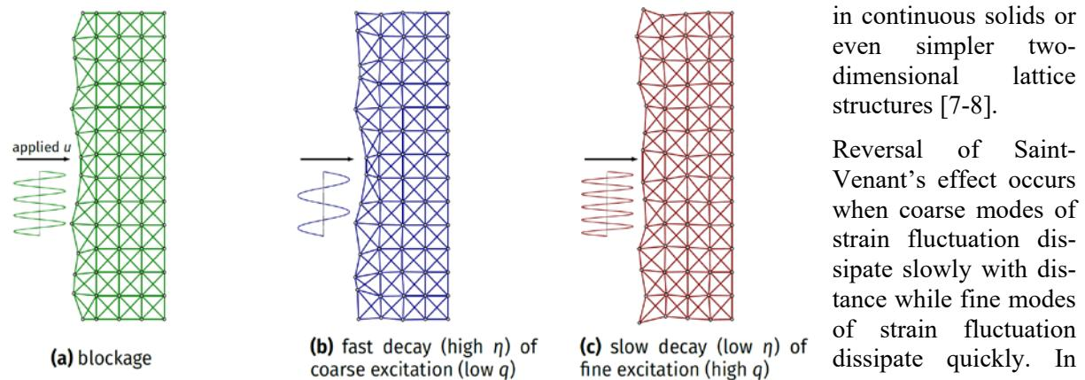
addition to exhibiting these two scenarios, RSV lattices are able to completely block some modes of strain fluctuation at the surface (Figure above).
