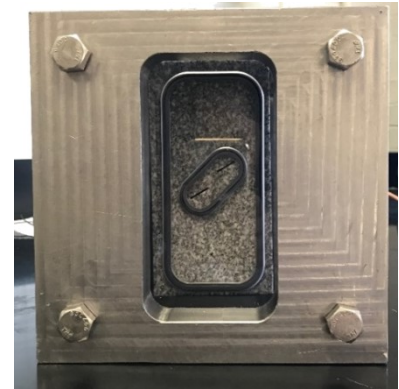
Figure 3. a) Scheme of the newly-designed pressure enclosure showing its different parts (b) front view of the pressure enclosure
