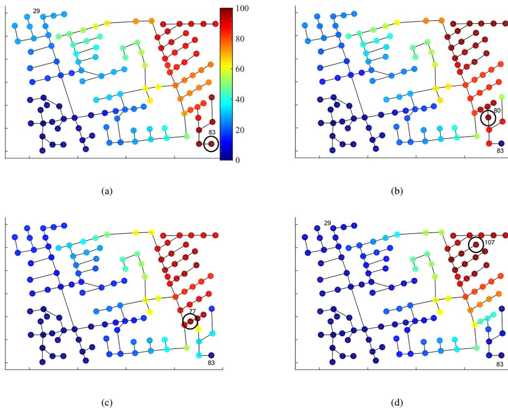
Figure 11: A gravity representation of the total eliminated index,  $I_{Te}$ , for IEEE 123-bus system.: (a) There is no ESS; (b) ESS installed at node 83 and rated for 6 kVA; (c) ESS installed at node 83 and rated for 13 kVA; and (d) ESS installed at node 83 and rated for 28 kVA.
