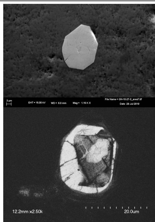
Figure 4: Backscatter electron image (top) and CL (bottom) of a euhedral zircon within the impact melt. CL shows that this is actually a zoned and irregular zircon with a very thin euhedral rim. We suggest that this formed by a small amount of new zircon growth in the impact melt on top of an existing older inherited zircon.
