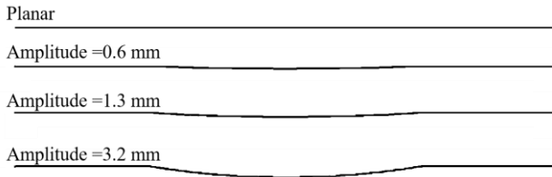
Fig. 6. A schematic of surface profiles for the prepared samples; from top to bottom (planar, G_.025, G_.05, G_.125), respectively.
