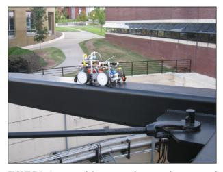
FIGURE 2 A smart mobile sensor used to assess the integrity of a bridge. Photo by Yang Wang used with permission.
