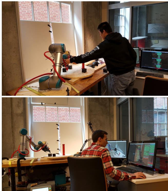
Fig. 1: Users interacted with the CoSTAR system in different ways. Left: a user positions the robot to teach it a new waypoint. Right: a user fine tunes part of a tree using the BT-based user interface.
