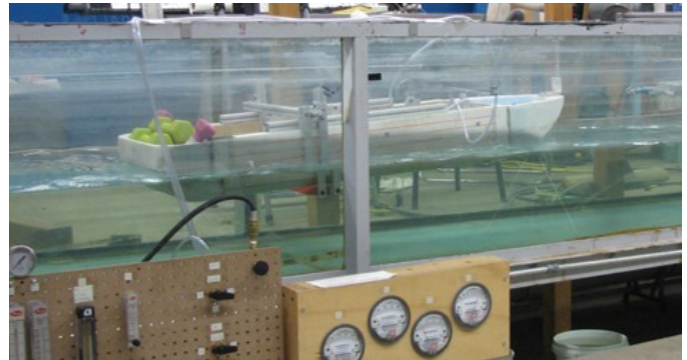
Fig. 5 Air-cavity hull tested in water channel
