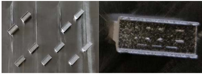
Figure 3. Five sets of Samples X and Y on the build plate (left), Zoomed view of the sample Y showing the single tracks(right).
