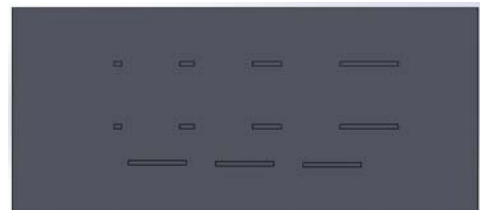
Figure 2. Top view of the single tracks of length 0.25, 0.5, 1 and 2 mm arranged in sample Y.
