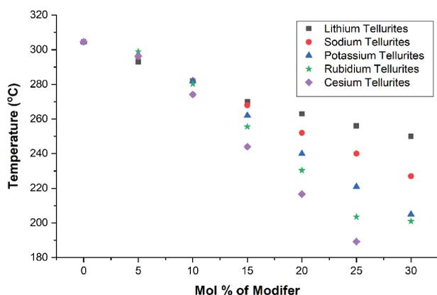
Figure 3.  $T_g$  of the alkali tellurite family with 5–30 mol% modifier. The  $T_g$  of pure TeO<sub>2</sub> is also plotted [Colour available online]
