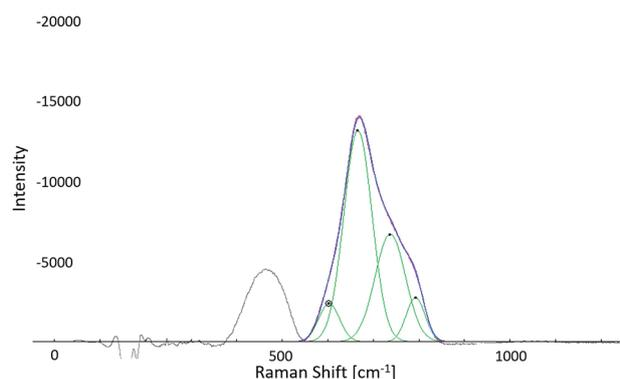
Figure 6. 10 mol % BaO.TeO<sub>2</sub> fit showing the deconvoluted peak positions. The two peaks on the left correspond to four coordinated units while the right two peaks are three coordinated. X-axis is Raman shift [cm<sup>-1</sup>] and the y-axis is intensity [Colour available online]
