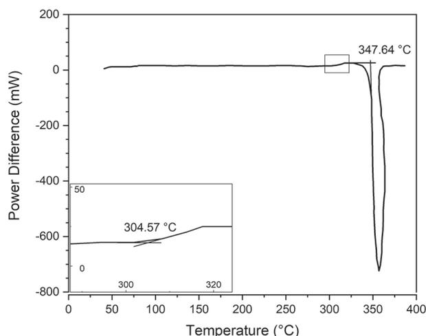
Figure 4. DSC output for amorphous TeO<sub>2</sub>. 305±3°C is the measured  $T_g$  and 348±3°C is the measured  $T_x$
