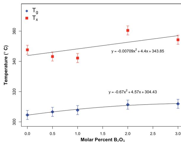
Figure 2.  $T_g$  and  $T_x$  of boron tellurites which were used to extrapolate the  $T_g$  and  $T_x$  of pure  $\text{TeO}_2$  using polynomial fits. Data points for the pure  $\text{TeO}_2$  results have since been added [Colour available online]
