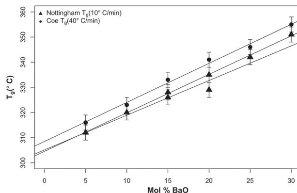
Figure 7. The  $T_g$  of barium tellurite glasses with a linear trend estimating the  $T_g$  of pure TeO<sub>2</sub>. Results were obtained using two different DSCs and ramp rates as described in the thermal measurements section
