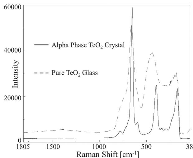
Figure 5. Raman spectra of amorphous TeO<sub>2</sub> glass and the  $\alpha$ -phase TeO<sub>2</sub> crystal
