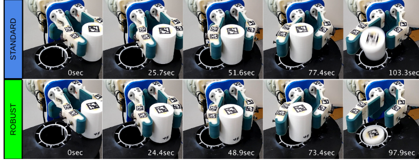
Fig. 6 Demonstration of STANDARD and ROBUST plans on the three-finger Model-O underactuated hand [25] for a peg-in-the-hole task.
