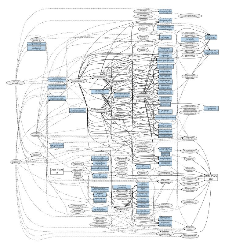
Fig. 11: Event flow graph of ONOS with core service components and several apps (*i.e.*, acl, fwd, mobility, dhcp, and dhcprelay). Blue rectangles represent event listeners and packet processors, gray ellipses represent API methods, bold edges represent event dispatches, and dashed edges represent API calls. (For simplicity, event types are reduced to a single edge of the event type's respective event kind.)
