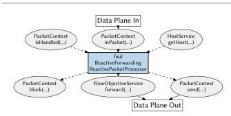
Fig. 6: Event flow graph of fwd's packet processor. Blue rectangles represent event listeners and packet processors, gray ellipses represent API methods, and dashed edges represent API calls.
