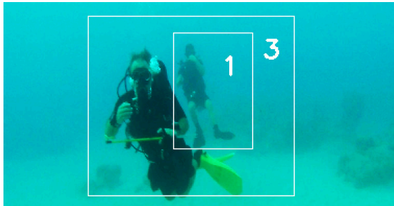
Figure 2: Exemplary output of our tracker on an underwater scene with multiple divers present. Two divers are detected and determined to belong to tracks “1” and “3.”
