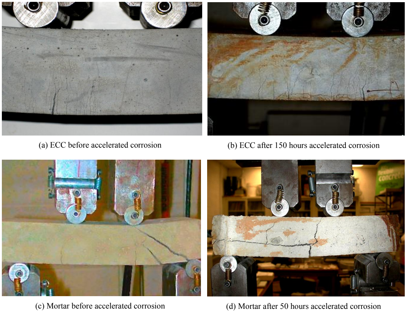
Figure 13 The damage tolerant behavior of ECC prolongs the corrosion propagation period and protects the beam element from failure, when subjected to an accelerated corrosion environment. After Sahmaran et al. (2008)
