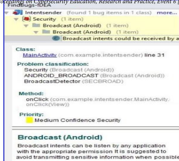
Figure 3: Broadcast intent detected by FindSecurityBugs
