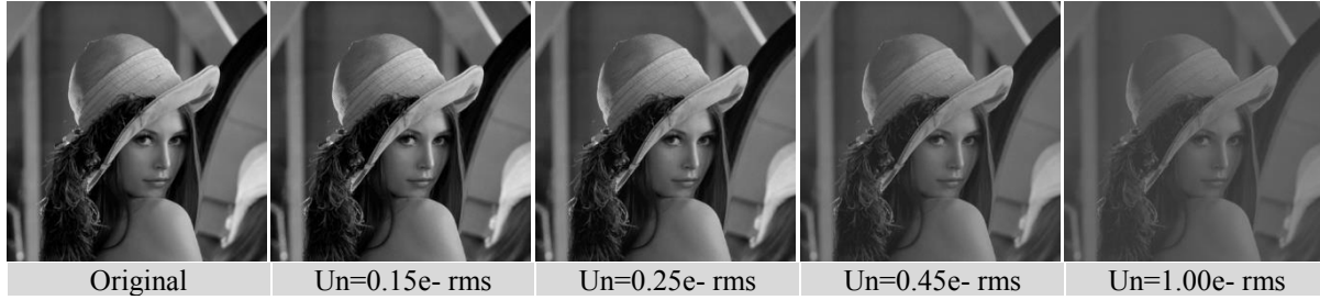
Figure 1: Simulated images for a 2-bit QIS with different read noise ( U_n ) levels. The quanta exposure H=0.3e^- and the oversampling factor M=10,000 , equivalent to 3,000 photons/pixel in average.
