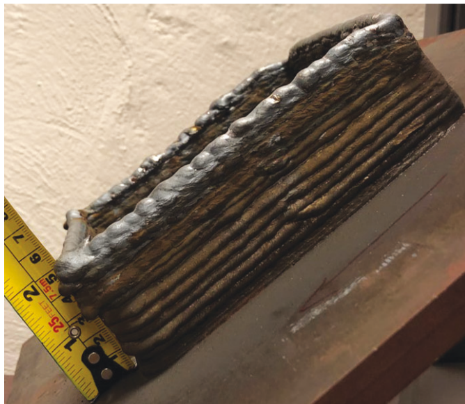
Figure 4: Initial build of 45° part
