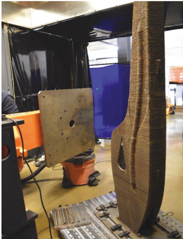
Figure 1: Example of a large part created using a WAAM process from [4].
