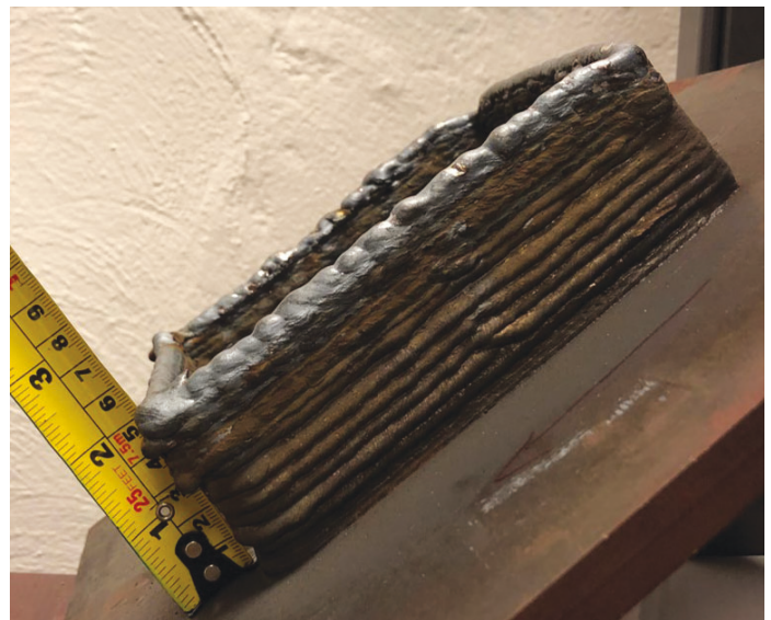
Figure 10 - Initial 45-degree part results. Note the bumpiness in the vertical sections while the horizontal sections had a much smoother surface.
