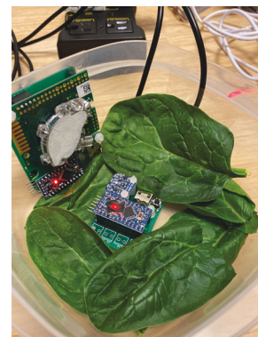
Figure 3. A mini-biosphere in preparation, containing spinach, a carbon dioxide sensor, and light sensor. The container would later be sealed using plastic wrap and rubber bands.
