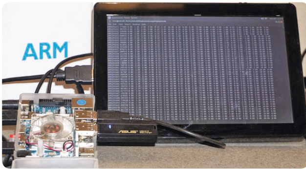
FIGURE 1 The Odroid-XU3 used as a prototype in this article. The processor is a Samsung Exynos 5422 with eight cores, and it was built using ARM big.LITTLE technology. The operating system is Ubuntu 15.04.
