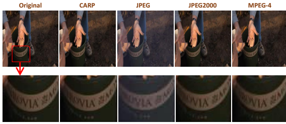
Figure 10. One frame of reconstructed YouTube videos. Left to right: original, CARP, JPEG, JPEG2000, and MPEG-4. Compression ratio is set to 30.
