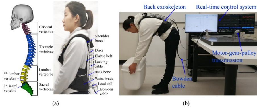
Fig. 15 (a) The spine-inspired back exoskeleton leverages on a hyper-redundant continuum mechanism. Thanks to its compliance, this wearable robot provides assistive force while being conformal to the anatomy of the human back and unobtrusive for natural motion. (b) A healthy subject wearing the back exoskeleton to perform stoop lifting of a 15 kg load. The spine continuum mechanism is powered by a tethered actuation platform via Bowden cable transmission.
