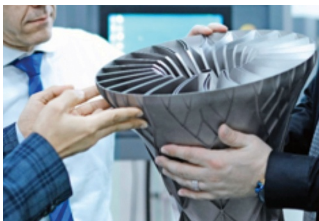
A Ti-6Al-4V turbine cooling test bed size, measuring 365 × 365 × 320 mm with a complex internal structure, is able to be additively produced on a Farsoon Technologies FS42IM system in one piece. (Courtesy of Farsoon Technologies.)
