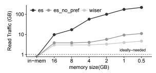
Figure 3: **Read Traffic of Search Engines** This figure shows read I/O traffic of various search engines as the size of memory decreases. es: Elasticsearch, es\_no\_pref: Elasticsearch without prefetch. Note that serving queries leads to only read traffic. The ideally-needed traffic assumes a byte-addressable storage device.
