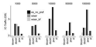
Figure 10: **Decomposed Traffic Analysis of Phrase Queries** The bars show the ideal traffic sizes for each engine, assuming the storage device is byte-addressable. The sizes were obtained by adding counters to engine code.
